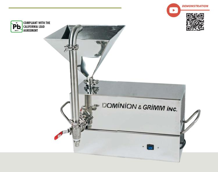
Mixer holding up to 2 gallons of maple syrup. 3/4 hp - 110 Volts electric motor. 1" Brass "Oberdorder" gear pump. All stainless steel plumbing on ferrules with fittings fully removable for a quick cleaning of the tank and the plumbing.
