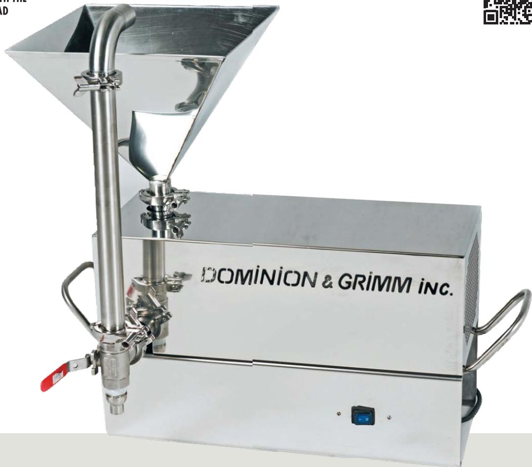
Mixer holding up to 2 gallons of maple syrup. 3/4 hp - 110 Volts electric motor. 1" Brass "Oberdorder" gear pump. All stainless steel plumbing on ferrules with fittings fully removable for a quick cleaning of the tank and the plumbing.
