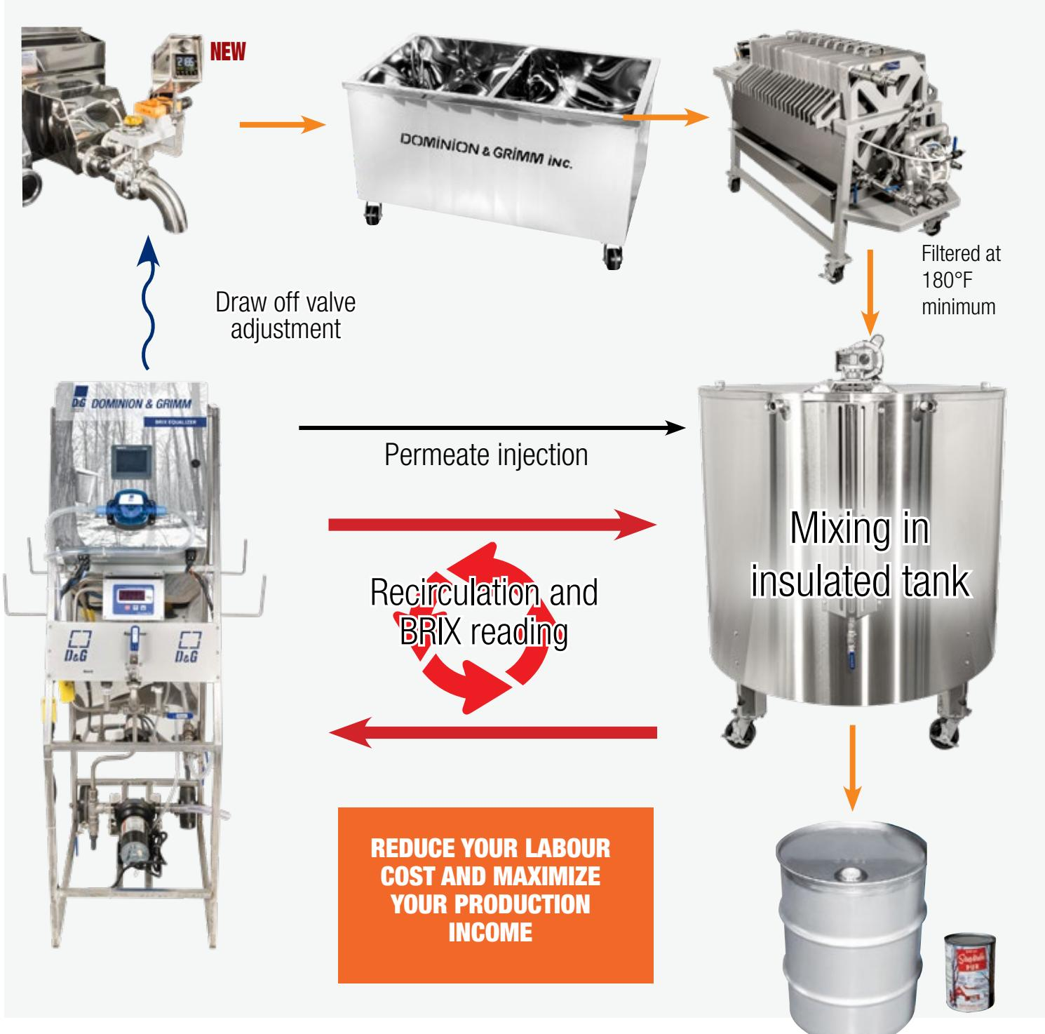
~~~~~ → Adjustment of the draw-off temperature value of the evaporator draw off according to the BRIX degree to be reached in the mixing tank
